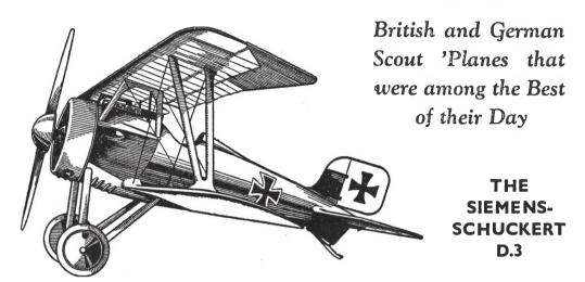
THAT the German aircraft designers of 1918 were well ahead with their ideas is evident from the streamlined appearance of this Siemens-Schuckert scout with its up-to-date "V" type racing strut. Other notable features of the design were the balanced ailerons on both planes and the balanced rudder and elevators. Its stumpy fuselage made the D.3 a somewhat tricky machine to handle, but once its habits were known its extraordinary manœuvrability endeared it to experienced pilots
