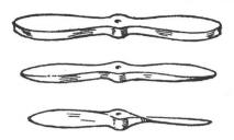
Fig. 3.—Three stages in the carving of an airscrew from a wood billet
